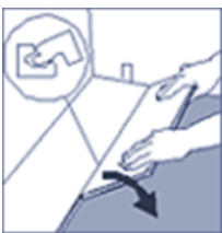
Fig 3. Fold / Angle the plank down. During the angle process make sure the planks are tight against each other. Afterwards press down or slightly tap down at the short end or long edge of the installed plank till its flat. No major force is or required, use a tapping block or piece of softwood to avoid edge damage.
