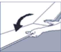
Fig 2. Second plank, first row angle long side & angle short end into place gently and tight to the short end of first plank. Light hand pressure or a lengthways tap maybe required to secure tightly. Please make sure both long edges and short ends are tight with no visible gaps.
