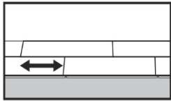
Fig 7. General distances between short ends. Minimum distance between short ends of planks in parallel rows shall not be less than 300-500 mm. This improves the stability of the floor.
